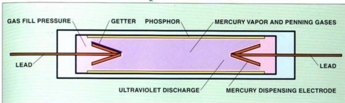
In the cold cathode fluorescent lamp construction it typically includes a hollow glass cylinder that has been coated on the inside with a phosphor material composed of rare earth elements such as zinc silicate and various types of halophosphates.
